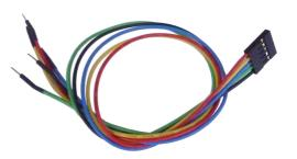
This 12" (300mm) long jumper cable is composed of 5 conductors with a 0.1" (2,54mm) spacing female socket on one end and machine pins on the other end.
