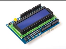
The *LCD Shield for Arduino* allows an Arduino board to visualize informations on an attractive LCD display with white text on blue backlight.
