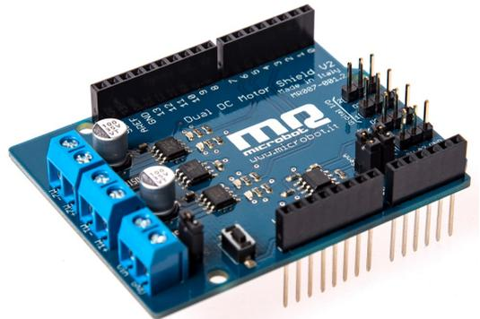
The *Dual DC Motor Shield V2* is a shield that has been projected to enable an Arduino board to drive two brushed DC motors or one 4-wire two-phase stepper motor, controlling the speed and direction of each one independently.
