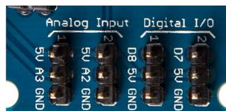
*Fig.1 – Digital and Analog ports*
