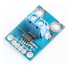
This board carries the Allegro's ACS711ELCTR-12B-T hall effect-based linear current sensor, which offers a low-resistance ( $\sim$ 1.2m $\Omega$ ) current path.
