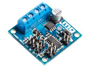
The Easy Motor Controller allows to control the direction and the speed of rotation of a DC motor through three different inputs: analog (potentiometer), radio control RC, I2C digital communication.
